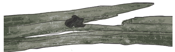
Figure 16.3 Glulam beam with a significant knot in the third lamella after a fire
