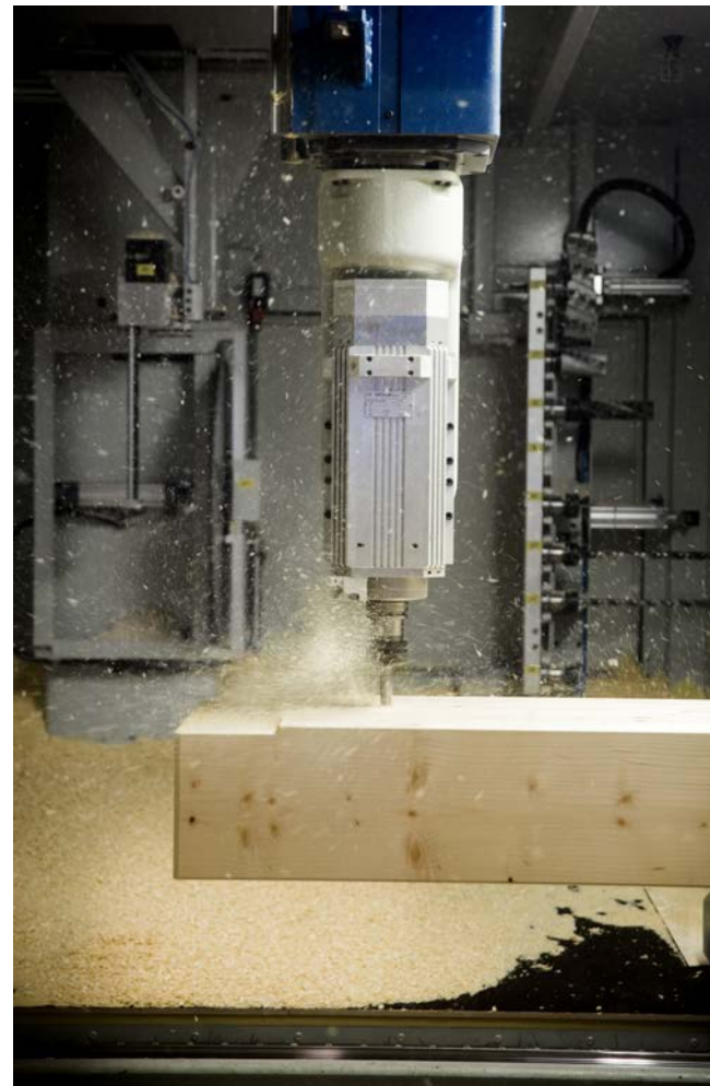
CNC machining of glulam beam.
