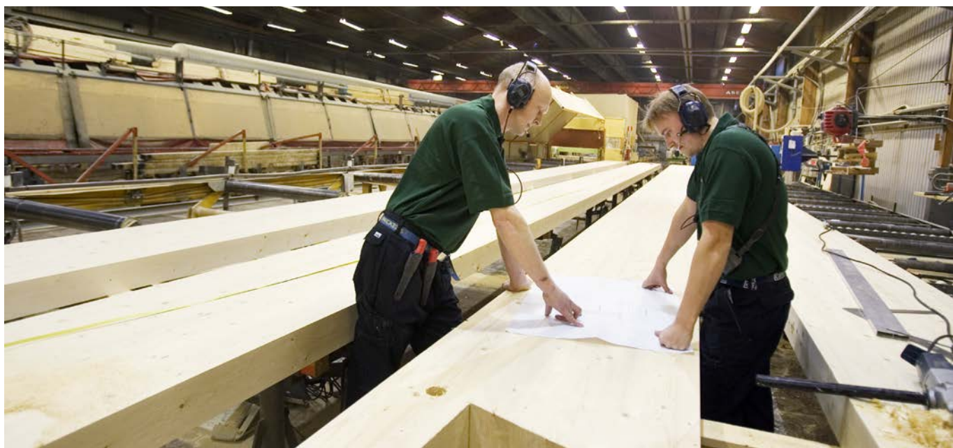
Glulam is produced industrially under controlled conditions. The photo shows the finishing of glulam beams.
