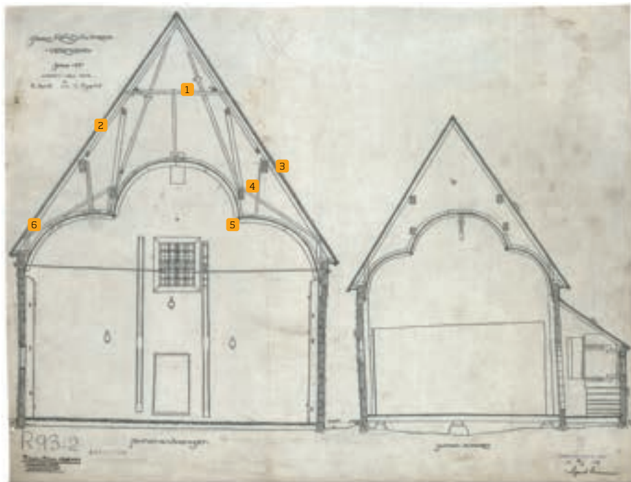
Roof with both purlins and trusses, drawing from 1909. 1. Collar tie. 2. Spar/rafter. 3. Purlin for roof. 4. Purlin for vault. 5. Decorative rope moulding. 6. Spur.
