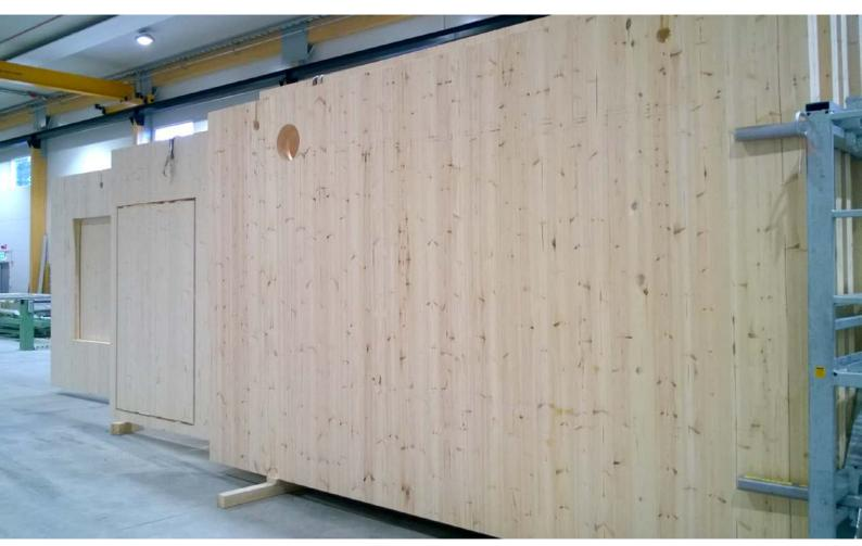
CLT panels reading for wrapping and delivery.
