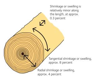
**Figure 2** Shrinkage or swelling in a softwood log from fresh to fully dry. Shrinkage or swelling in a piece of timber varies depending on how the growth rings are positioned in the wood. The smallest dimensional changes occur in wood where the growth rings are perpendicular with the face, known as vertical grain.
