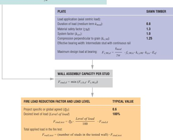
Figure 1: Establishing the magnitude of the structural load for a product assembly in EN fire test
