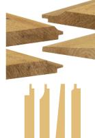
Timber is increasingly used for the exterior cladding of buildings of many different construction types. Both softwoods and hardwoods are suitable. Softwoods should generally be pressure treated with preservative, although Larch and Western Red Cedar can be used untreated if the sapwood is excluded.
