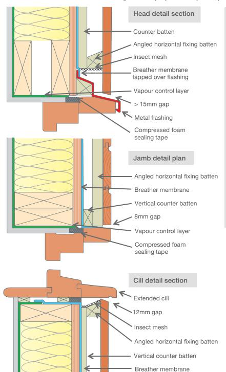
Typical detail of window in vertical tongue and grooved cladding. The drawings show a timber frame wall. Detailing will be similar with other forms of wall construction.
