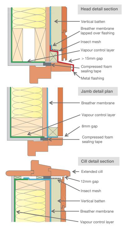
Typical detail of window in horizontal cladding. The drawings show a timber frame wall. Detailing will be similar for other forms of wall construction.
