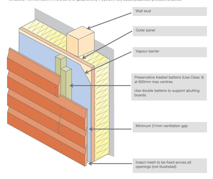
This drawing is for horizontal cladding fixed to a timber frame structure.
